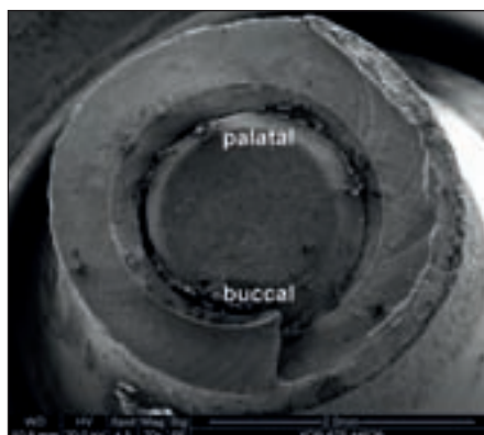
SEM image showing the fracture surface of a clinically failed dental implant
