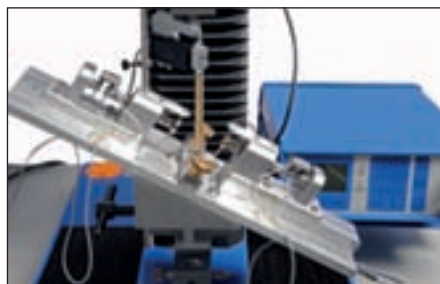
In vitro test setup for measuring micromotion between implant and abutment
