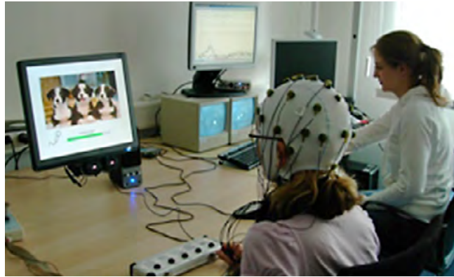
At this psychophysiological working station a subject is looking at an emotion inducing picture on the monitor. Her brain electrical activity, heart rate, skin conductance, speech and eye movements are measured. This multilevel approach can be used to examine the interaction of cognition and emotion.
