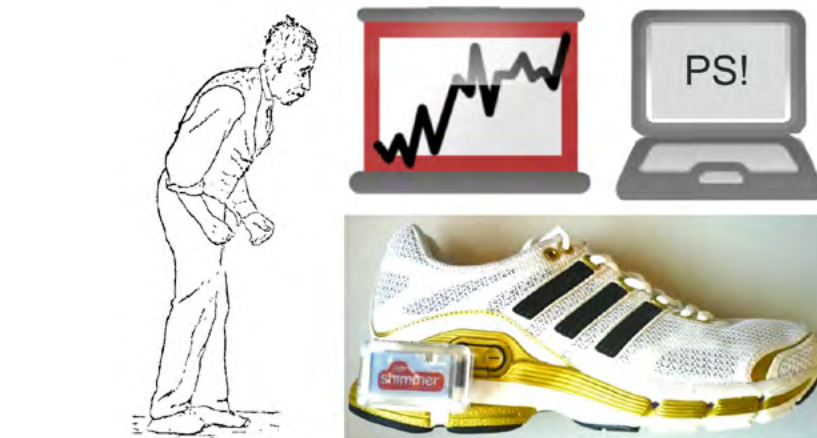
Gait impairment in Parkinson's syndrome (PS) can be detected using a sensor based movement detection system attached to a sport shoe. Motion data is classified using pattern recognition technique and provide objective information of gait impairment in PS
