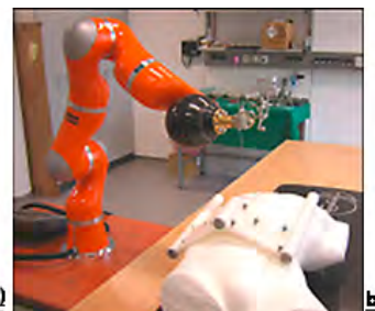
a) Concept of using robots in medical imaging and surgical interventions. [Kalender, 2007] b) Implementation of a KUKA light weight robot in experiment in a navigation and robot-assisted intervention at the IMP
