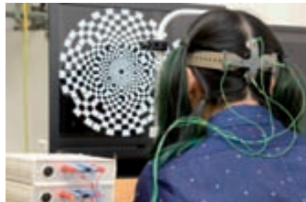
Experimental set up for measurements of multifocal visual evoked potentials in human observers.
