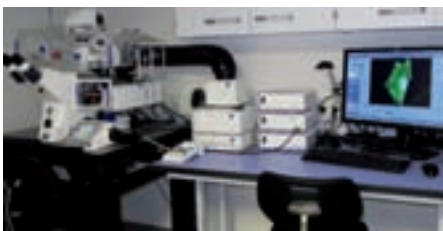
Zeiss Life Cell Imaging System Axio Observer Z1 with incubation unit for the morphologic and toxicologic observation and quantification of eukaryotic cells.
